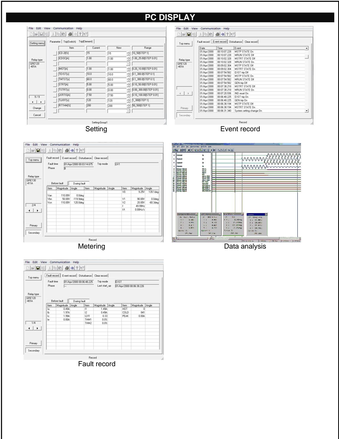
Figure 4 - Relay Setting and Monitoring System - PC Displays
